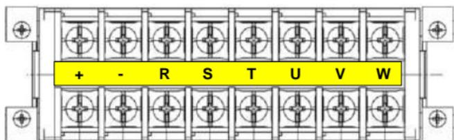
Fig C.5 Wiring terminals of 4T models for inverters  $\leq 2.2\text{kW}$
