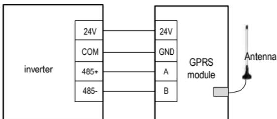
Fig A.2 Connecting the GPRS module to the inverter
