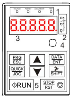
Fig 4.2 Keypad diagram for inverters  $\geq 4\text{kW}$
