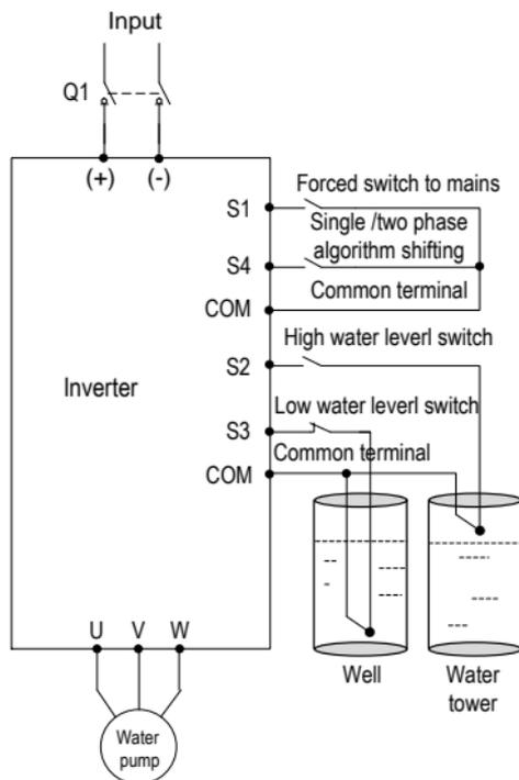
Fig 3.3 Standard wiring diagram
