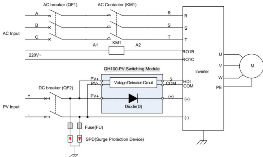
Fig C.1 Inverter power frequency & PV switching solution
