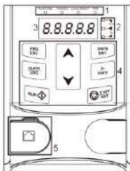
Fig 4.1 Keypad diagram for inverters  $\leq 2.2\text{kW}$
