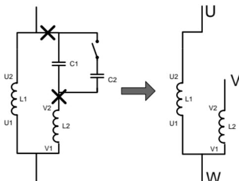
U1 and V1 are the common terminals of the windings. Connect them to the output terminal W of the solar pumping inverter. Connect U2 to the output terminal U of the inverter. Connect V2 to the output terminal V of the inverter. (**Note:** Use the screws equipped with the inverter.) Connect S4 of the inverter to COM in short circuited manner.
